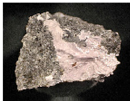
Pinkish-white Kimuraite-Y \text{Ca}(\text{Y,Nd})_2(\text{CO}_3)_4\cdot 6\text{H}_2\text{O} from Japan contains yttrium and neodymium. Field of view 1 cm.
